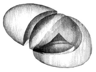
Figure 2. The common optimal space between the two performance loci obtained through the Boolean operation of intersection
